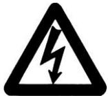
Lightning flash with arrowhead symbol within an equilateral triangle warns user to the presence of uninsulated "dangerous voltage" within the product's enclosure of such value that it can result in electrical shock.
